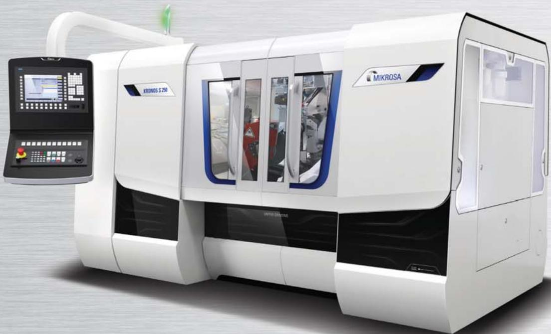
Are you looking for the most efficient way to grind your small, high-precision workpieces? Then you have found the new KRONOS S by MIKROSA! This compact and versatile centerless grinding machine with an infeed length of 120 mm or 245 mm combines maximum speed with the highest quality requirements. The machine's broad technology spectrum extends from infeed grinding in single or multiple production to throughfeed grinding and oscillation grinding.
