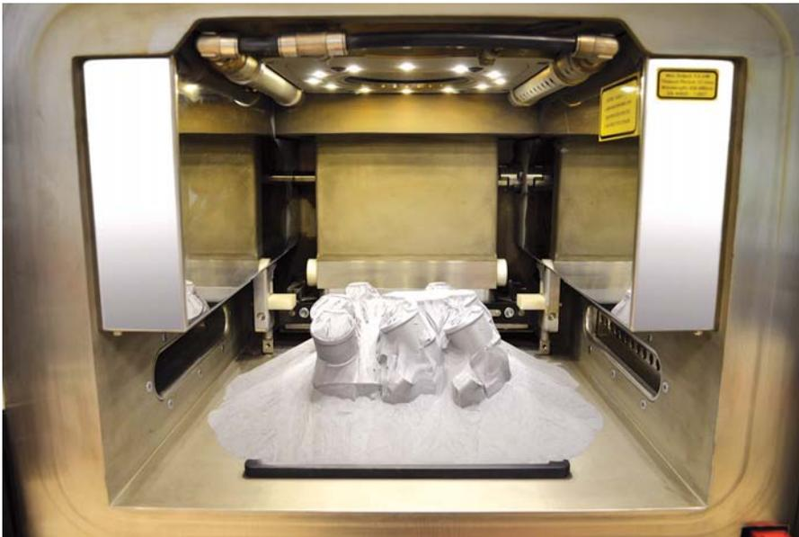
Mercedes-Benz Trucks produces complex metallic spare and special parts in top quality using a new 3D printing process. The photo shows the working cavity of the laser printer at whose centre a metallic thermostat cover has been produced for the first time using selective laser melting (SLM). When the work platform is raised, the powdered aluminium/silicon material moves to the side and the contours of the component become visible.
